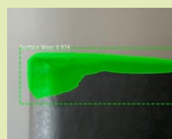
Clearance surface wear
