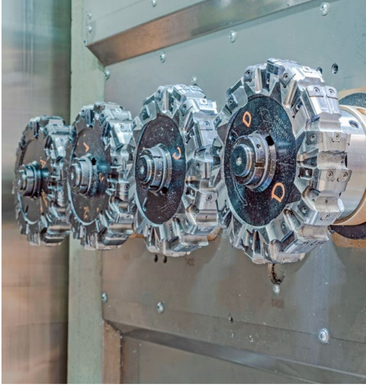
Quadruple application of disc milling cutters on control arms. The solid cutting surfaces provide an indication of the high drive power required (Photo provided by ELHA)
