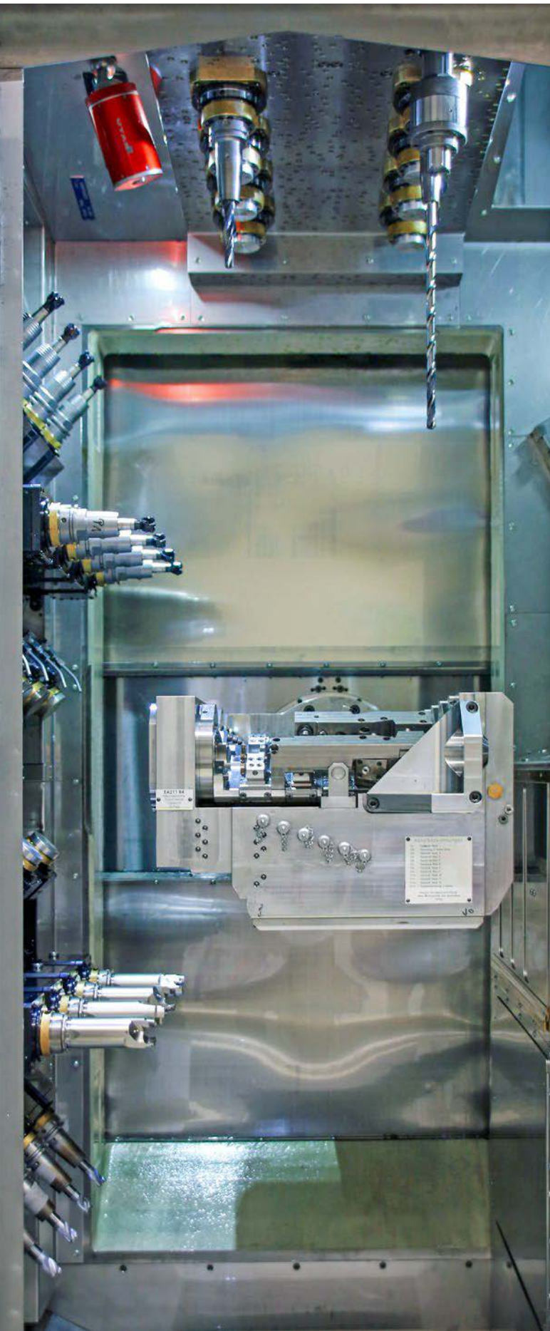
Arrangement of four step drills on the right-hand side of the working area of a production module (Photo provided by ELHA)
